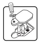
4. Replace the battery cover and tighten the screw to secure.
